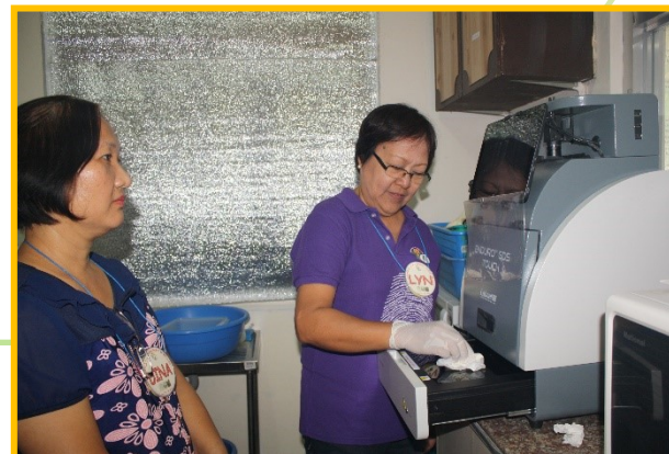
Viewing of electrophoresed PCR products on gel via UV transillumination
